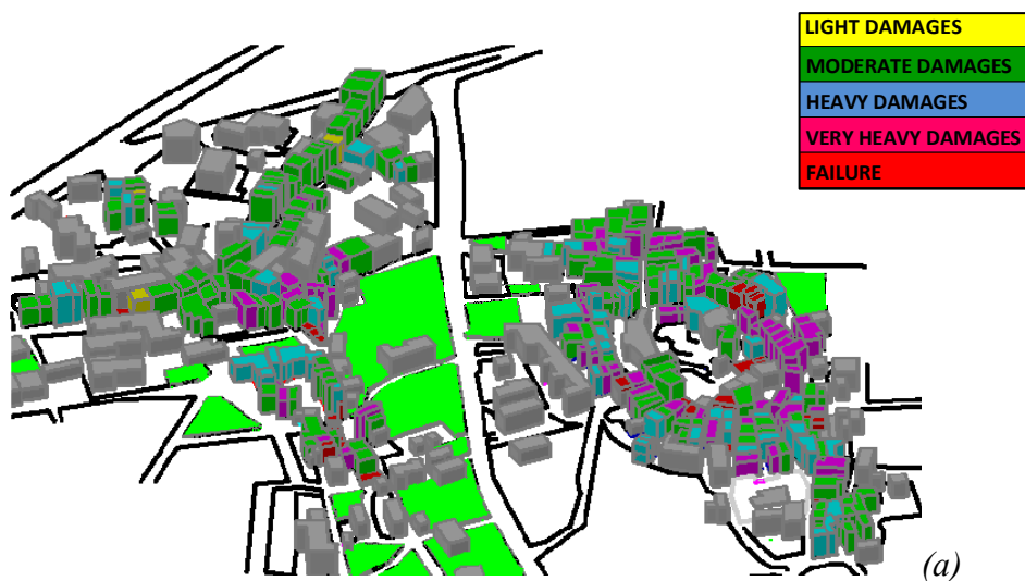
Figure 16. Comparison between forecast damages (a) and real ones (b) (continues).
