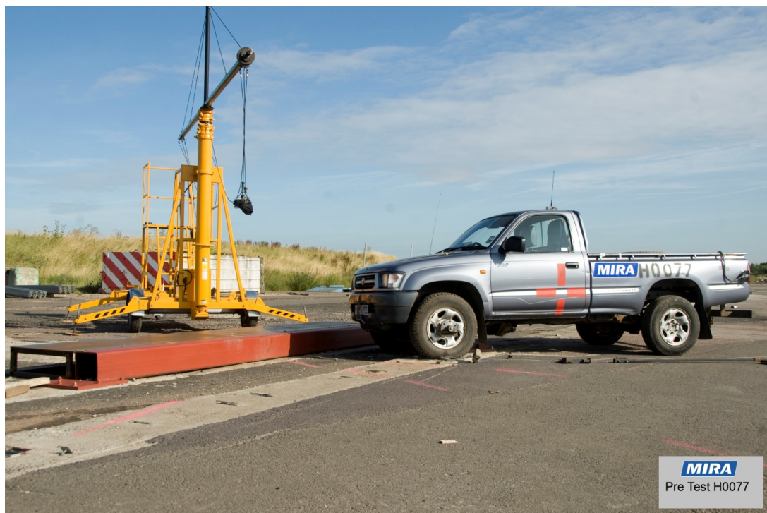
Figure 4: Kerb Impact test setup
