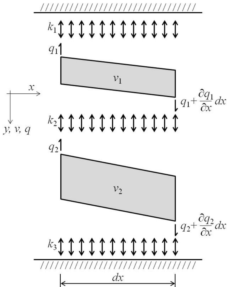
Figure 1. Positive sign convention for the instantaneous forces and displacements associated with a typical elemental length of the spring linked members in local coordinates.
