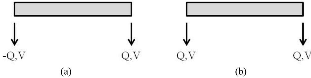
Figure 2. Positive sign convention for amplitudes of the nodal forces and displacements in (a) local; and (b) member co-ordinates.
