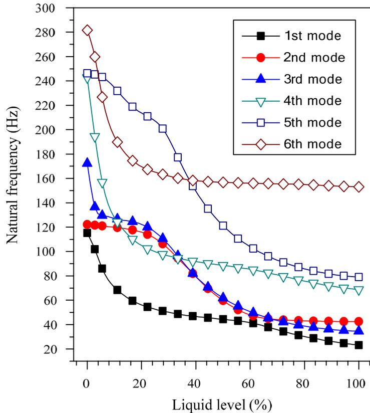
Figure 6: Effect of liquid level on the natural frequencies.
