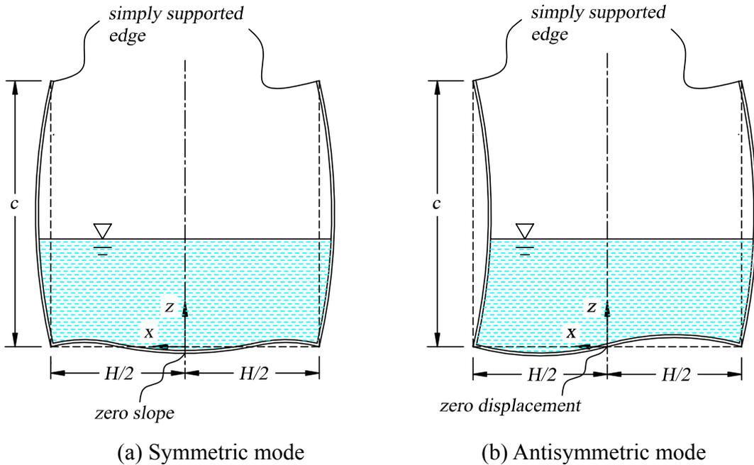
Figure 2: Mode category of a rectangular flexible open container partially filled with a liquid.
