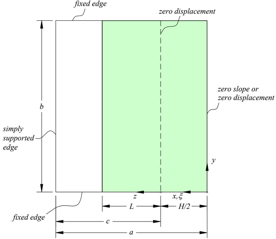
Figure 3: Theoretical model of a half of a rectangular flexible open container partially filled with a liquid.
