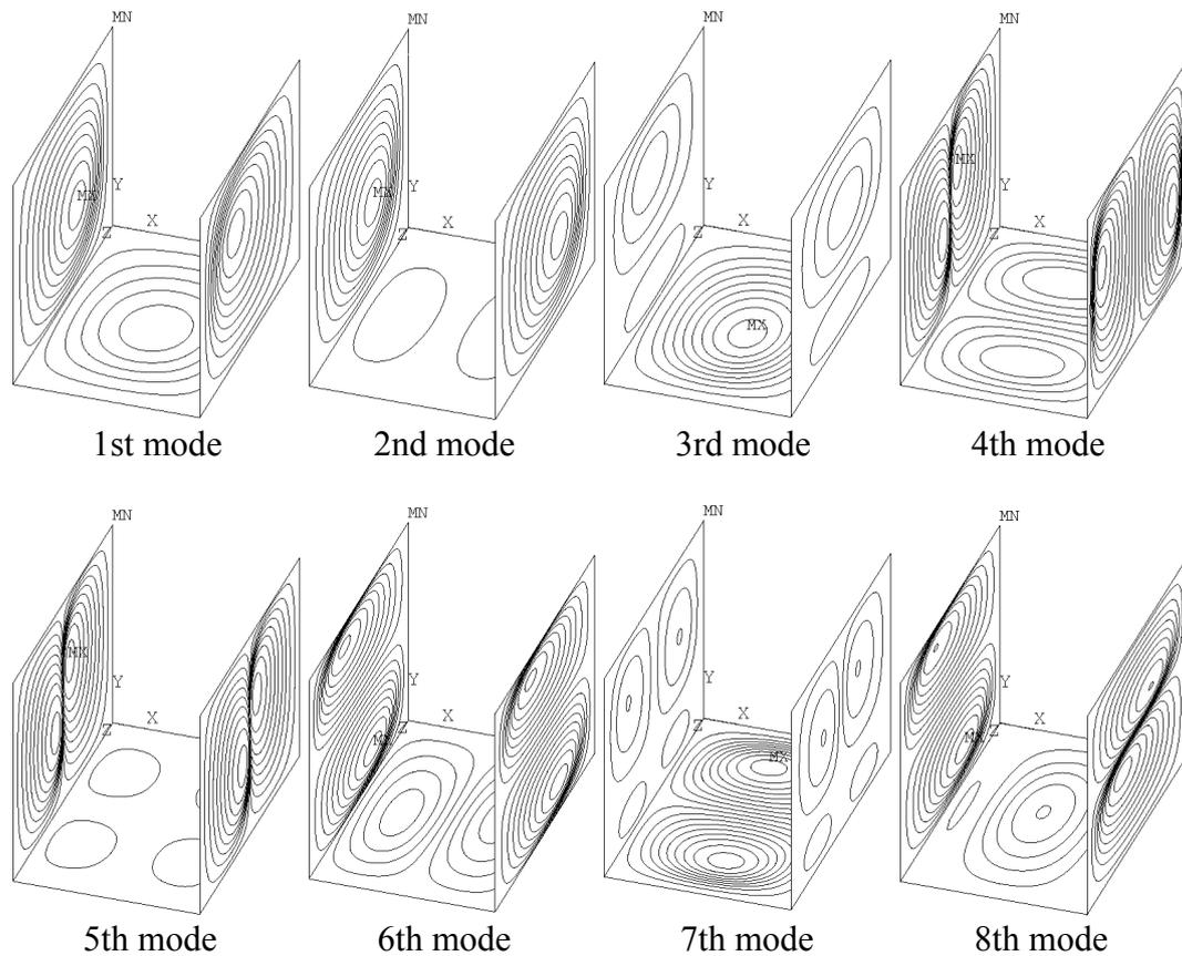
Figure 4: Mode shapes of a dry container.
