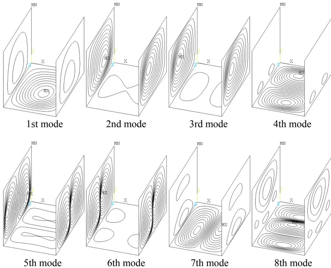
Figure 5: Mode shapes of a wet container with a half liquid level.
