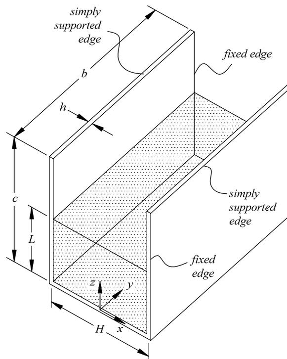
Figure 1: A rectangular flexible open U-type container partially filled with a liquid.
