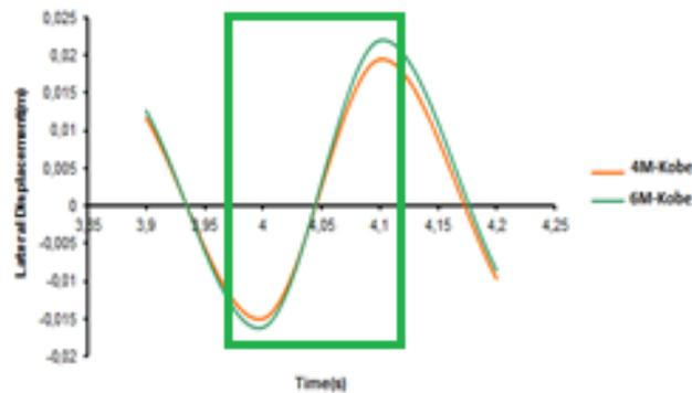
Figure 11. Maximum lateral displacements in Kobe's earthquake
