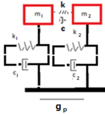
Figure 5. Schematic model of adjacent buildings with link having spring and dashpot damper
