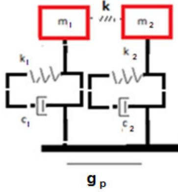
Figure 4. Schematic model of adjacent buildings with spring-link
