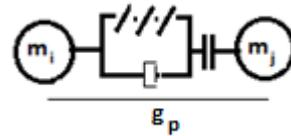
Figure 7. Schematic model of Kelvin-Voigt with gap
