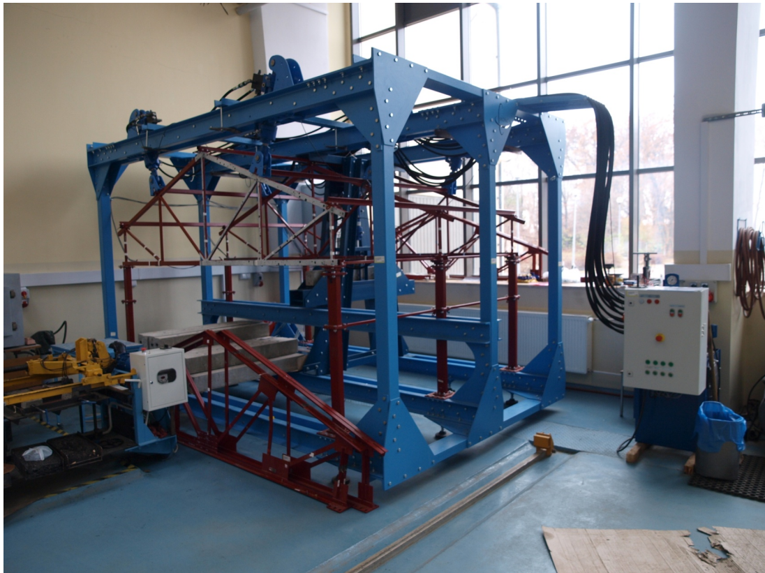
Figure 8. Test stand with tested truss inside during the experiment
