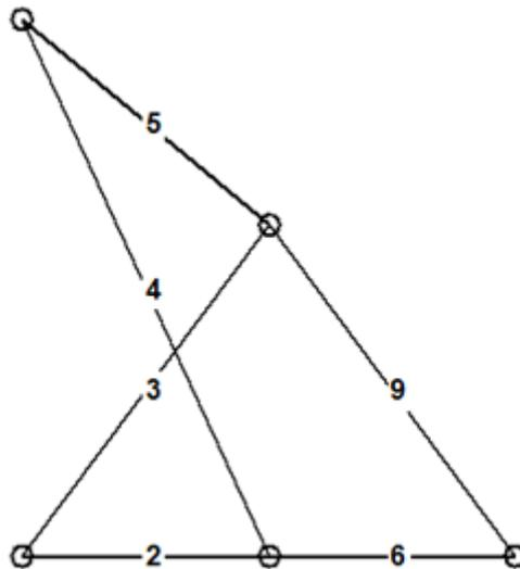
Figure 4: Optimal topology found in the size, shape and topology 11-bar truss optimization problem.
