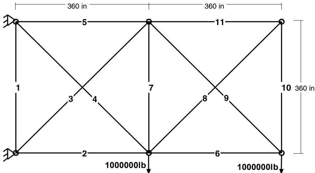
Figure 2: The 11-bar truss benchmark example: section 4.1.
