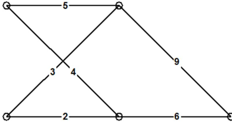
Figure 3: Optimal topology found in the size and topology 11-bar truss optimization problem.
