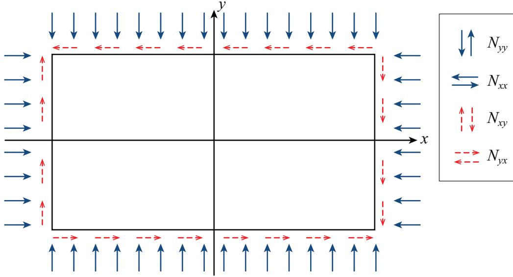
Figure 3: Rectangular plate subjected to in-plane forces.
