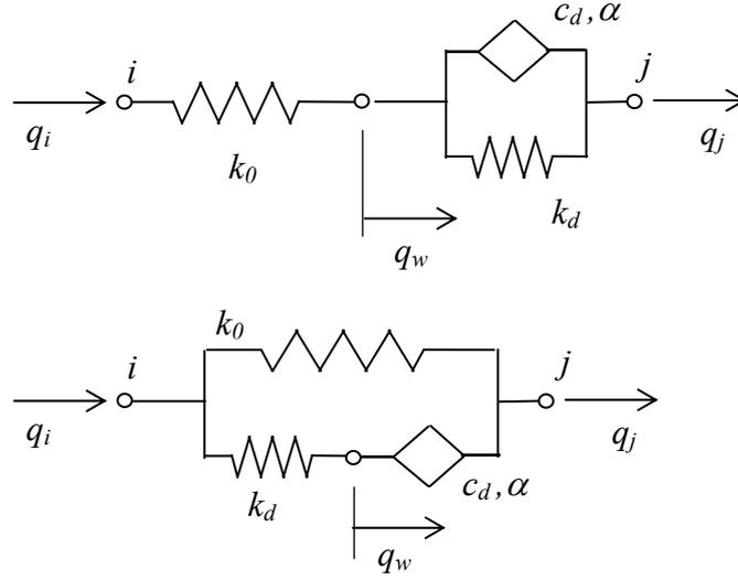
Figure 2: A four-parameter Kelvin (k4) and Maxwell (m4) models of damper.
