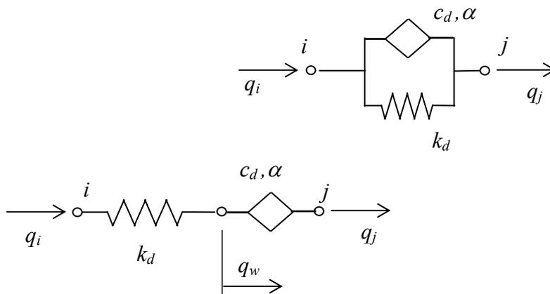
Figure 1: A three-parameter Kelvin (k3) and Maxwell (m3) models of damper.
