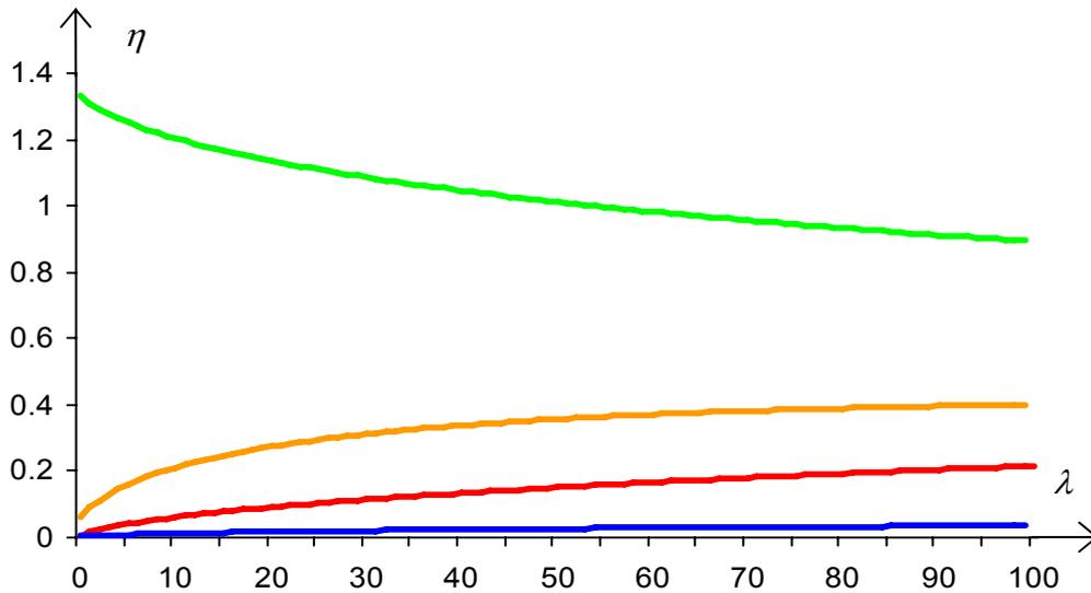
Figure 6: The function of loss factor for VE dampers – uniform data.
