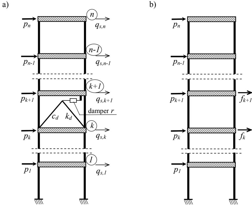
Figure 3: Diagram of frame with VE dampers.
