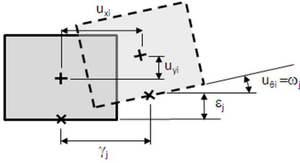
Figure 2: Block and contact kinematic variables.
