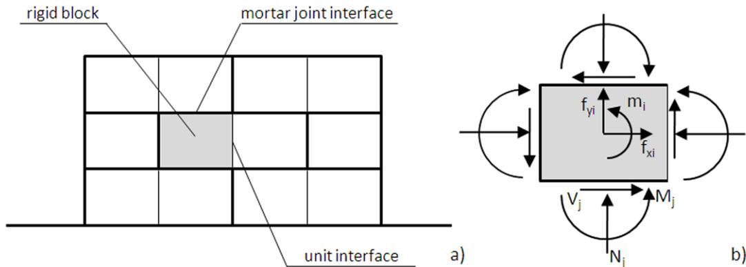
Figure 1: a) Proposed rigid block model with cracking units (masonry unit in thick line); b) Block and contact static variables.
