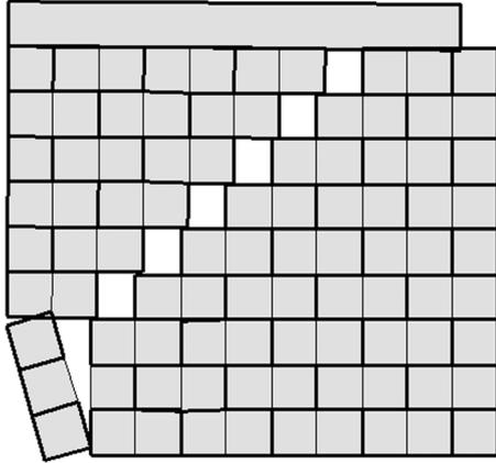
Figure 5: SW.200: Computed failure mode
