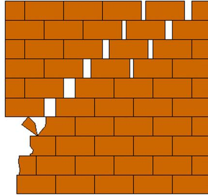
Figure 6: Experimental failure mechanisms for panel SW200 (adapted from Oliveira [9]).
