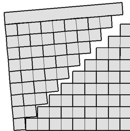
Figure 3: Rigid block model with cracking units of unconfined shear walls SW30 and SW200.
