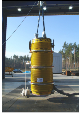
Figure 1: Model cask without impact limiter before drop test
