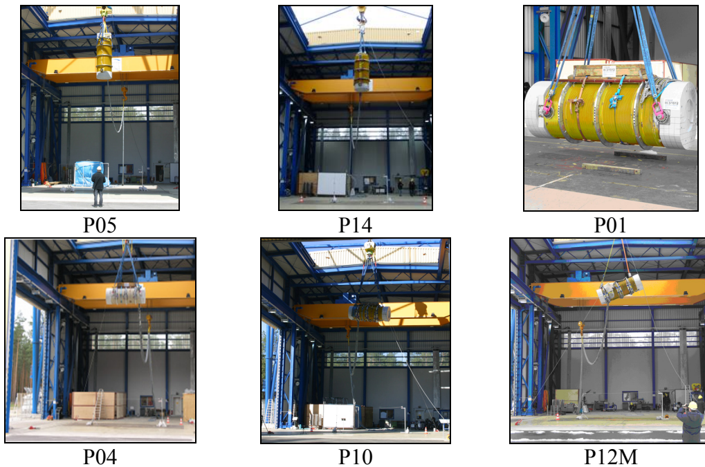
Figure 2: Model cask with impact limiter shortly before different drop tests
