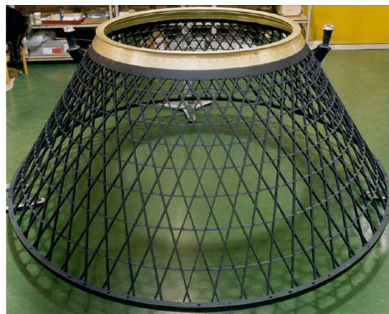
Figure 8 – Rocket structure composite unit.
