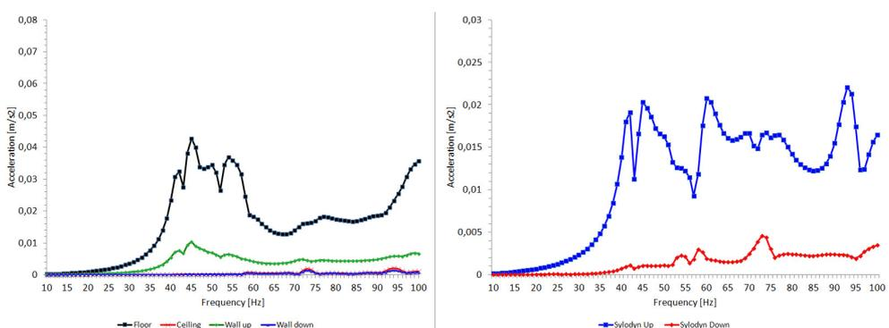
Figure 15: Case B widthwise. Acceleration magnitudes evaluated on the floor, ceiling, upper and bottom walls (left) and top and bottom of Sylodyn (right).
