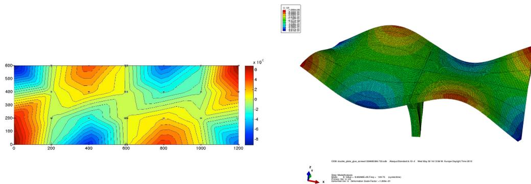
Figure 4: Eigenmodes, left: 6th measured, right: 7th simulated
