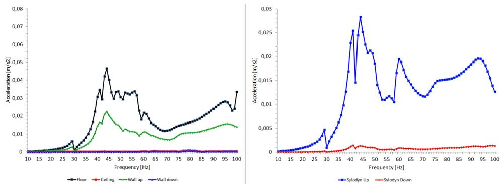
Figure 13: Case A widthwise. Acceleration magnitudes evaluated on the floor, ceiling, upper and bottom walls (left) and top and bottom of Sylodyn (right).
