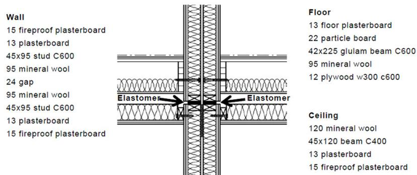
Figure 7: Separating wall junction with elastomer.
