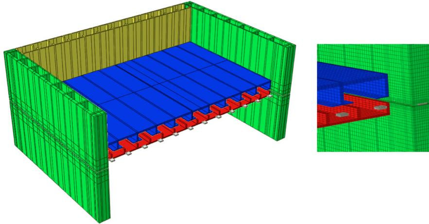
Figure 10: Case A: the beams being oriented widthwise.
