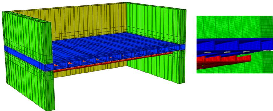
Figure 12: Case B: the beams being oriented widthwise.
