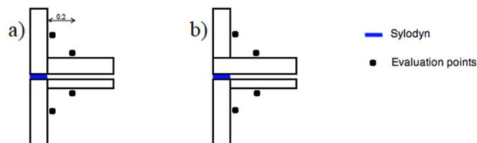
Figure 8: Two Syldyn positions; a) installed between the walls, b) installed between floor and wall.
