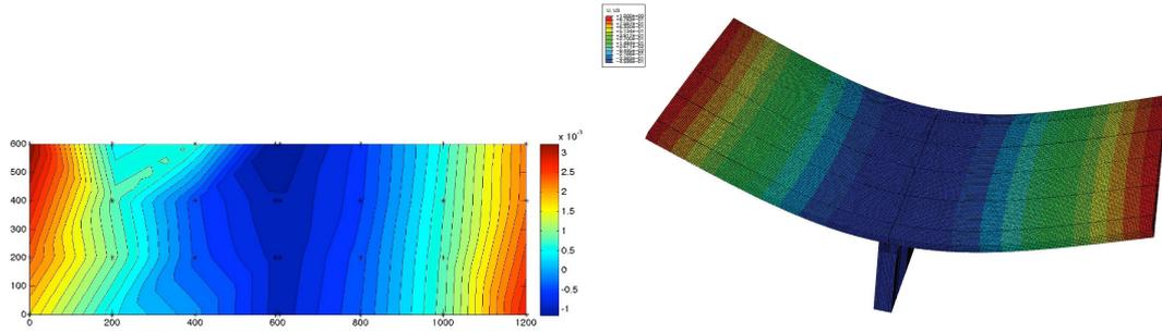
Figure 2: First eigenmode, left: measured, right: simulated
