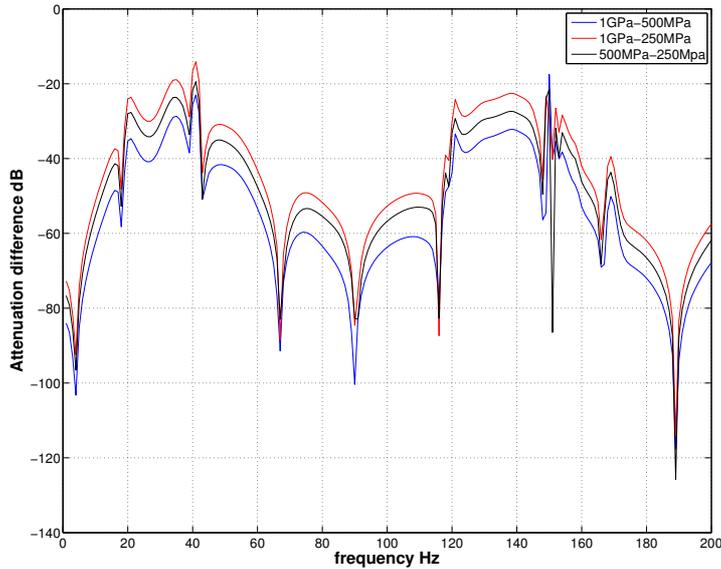
Figure 5: Attenuation differences dual plate cases 0 to 200 Hz
