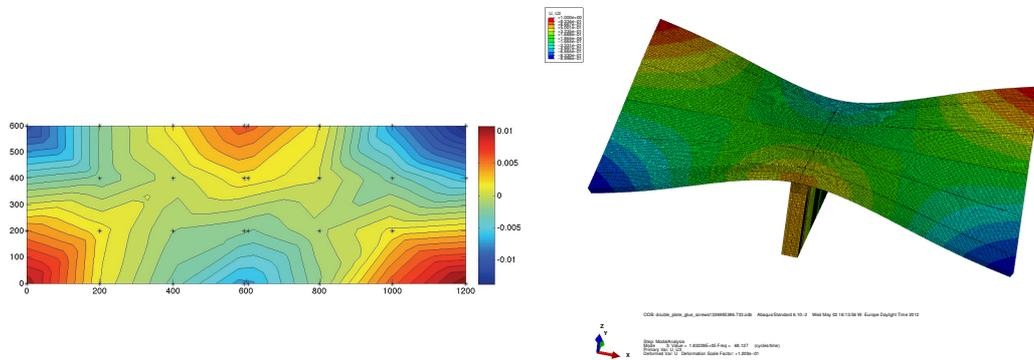
Figure 3: Third eigenmode, left: measured, right: simulated
