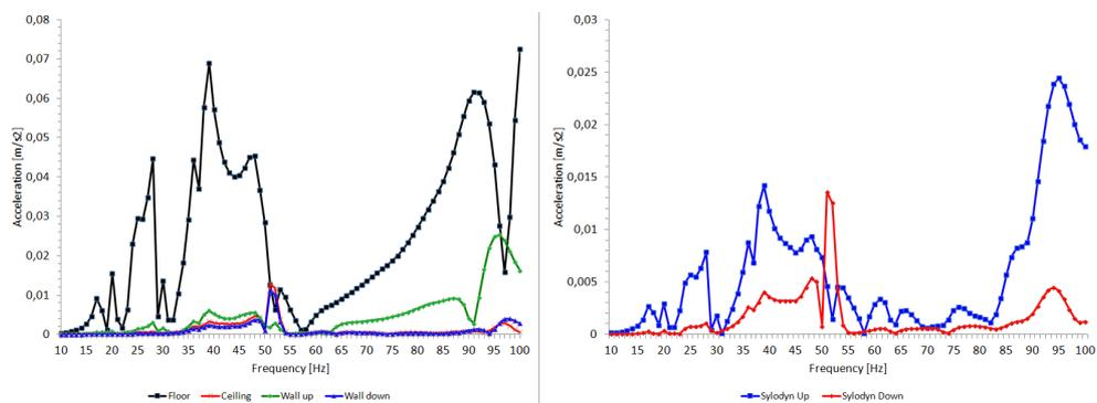
Figure 14: Case A lengthwise. Acceleration magnitudes evaluated on the floor, ceiling, upper and bottom walls (left) and top and bottom of Sylodyn (right).
