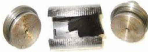
Figure 4: Axisymmetric deformation of a short model.
