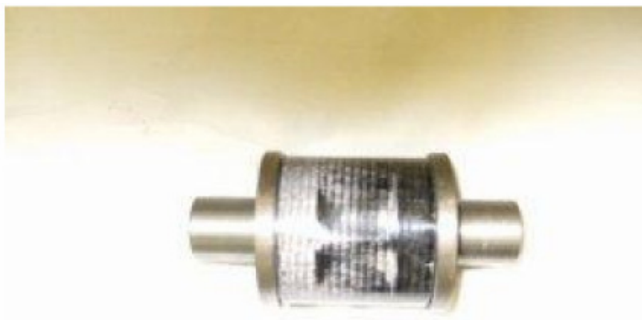
Figure 3: Inelastic buckling of a model.
