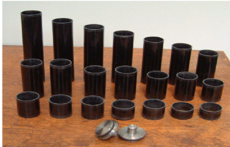
Figure 1: The PTSC carbon models and their end bungs
