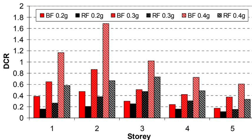
Figure 10. Maximum DCR values registered for the columns of each storey of the bare and retrofitted frames at different seismic intensity levels.
