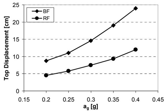
Figure 6. Maximum top displacement of the bare and retrofitted frames for different seismic intensity levels.
