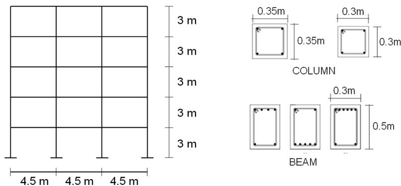
Figure 2. Elevation view of the RC frame and details of typical column and beam cross sections.
