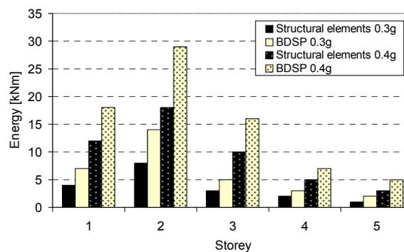
Figure 9. Energy dissipated by the structural elements and by the BDSP system at each storey of the retrofitted frame for different seismic intensity levels.
