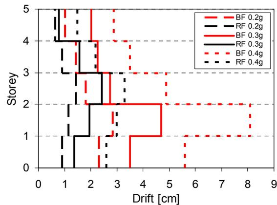
Figure 7. Storey drift profiles for the bare and retrofitted frames for different seismic intensity levels.
