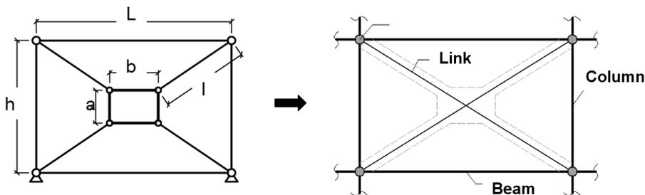
Figure 4. Geometric dimensions and schematic model of the BDSP system.
