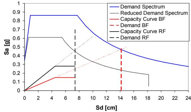
Figure 5. Demand spectra and capacity curves in AD format for the bare (BF) and retrofitted (RF) models.
