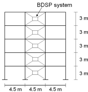
Figure 3. Elevation view of the RC frame equipped with braced ductile shear panels.
