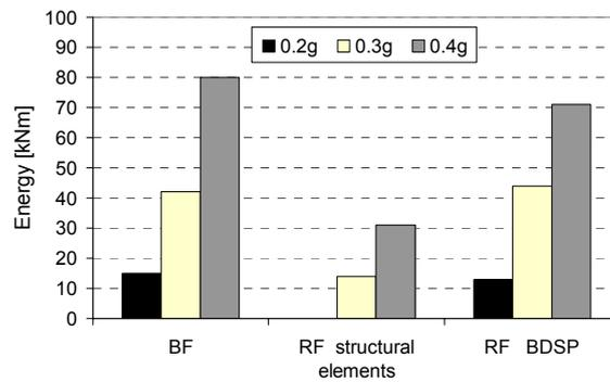
Figure 8. Energy dissipated by the bare frame and by the retrofitted frame (structural elements and BDSP system) for different seismic intensity levels.
