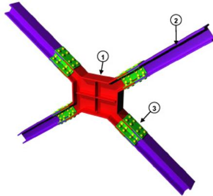
Figure 1. Schematic overview of the dissipative bracing system: (1) ductile shear panel, (2) braces, (3) bolted connection.
