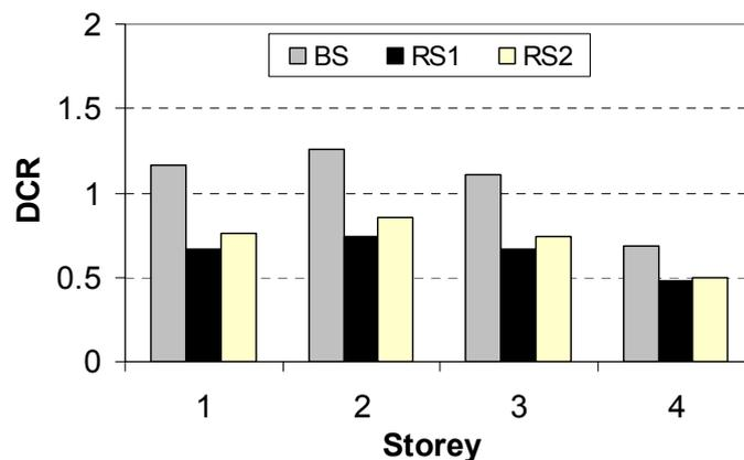
Figure 10. Maximum DCR values for the columns of each storey of the three investigated structures at  $Sa_g = 0.3g$  seismic intensity level.
