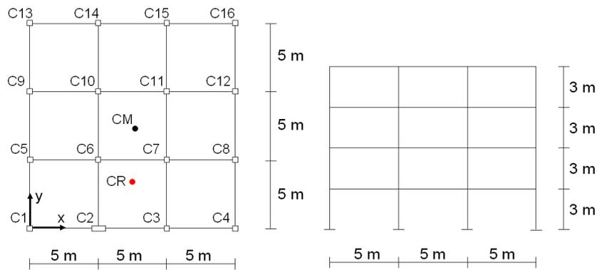
Figure 1. Schematic plan and elevation of the RC building and position of the centre of mass (CM) and the centre of stiffness (CR).
