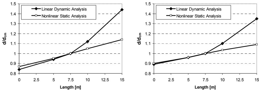
Figure 3. Normalized displacements at the top of the bare structure for linear dynamic analyses and nonlinear static analyses: x direction (left) and y direction (right).
