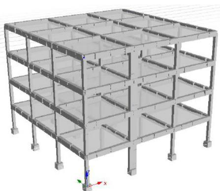
Figure 2. Three-dimensional view of the numerical model of the RC building.
