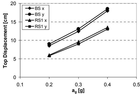
Figure 7. Maximum roof displacement in both directions for the bare and retrofitted structures as a function of the seismic intensity levels.
