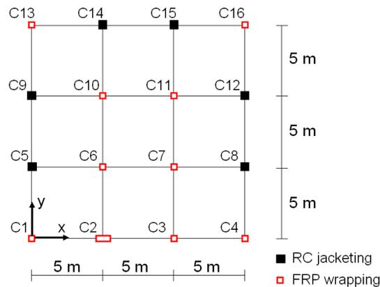
Figure 5. Schematic plan of the retrofitted structure RS1.
