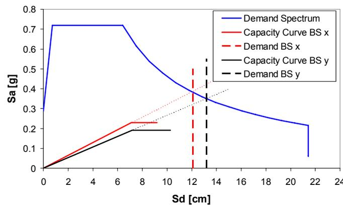
Figure 4. Demand spectrum and capacity curves in AD format at LSSD ( $S_{a_g} = 0.29g$ ) for the bare structure in the x and y directions.
