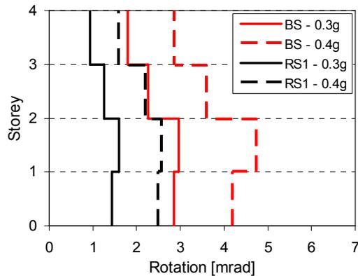
Figure 9. Storey rotation profiles for the bare and retrofitted structures at  $Sa_g=0.3g$  and  $Sa_g=0.4g$  seismic intensity levels.
