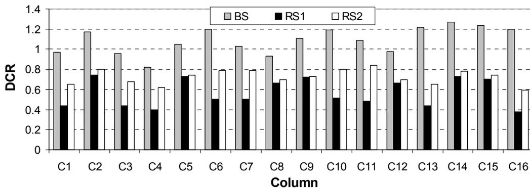
Figure 11. Maximum DCR values for the columns of the second storey of the three investigated structures at  $Sa_g = 0.3g$  seismic intensity level.
