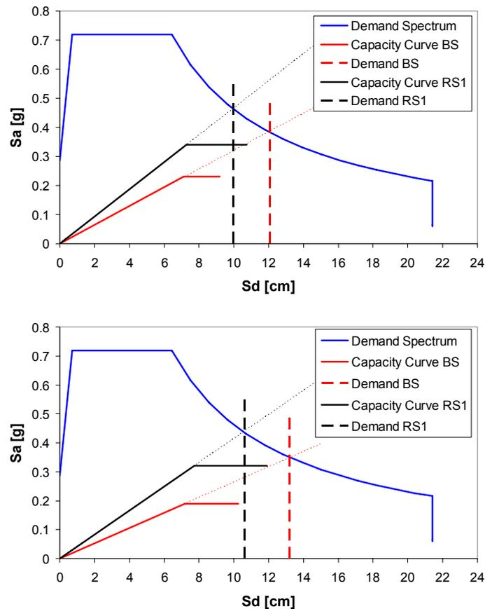
Figure 6. Demand spectra and capacity curves in AD format at LSSD ( $Sa_g = 0.29g$ ) for the retrofitted structure RS1: x direction and y direction.
