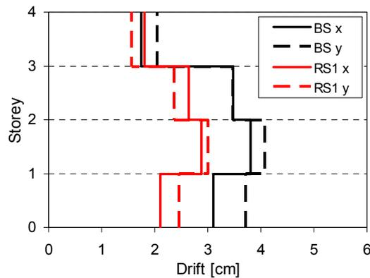
Figure 8. Storey drift profiles in both directions for the bare and retrofitted structures at  $Sa_g = 0.3g$  seismic intensity level.
