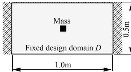
Figure 2: Fixed Design Domain  $D$  and Boundary Conditions
