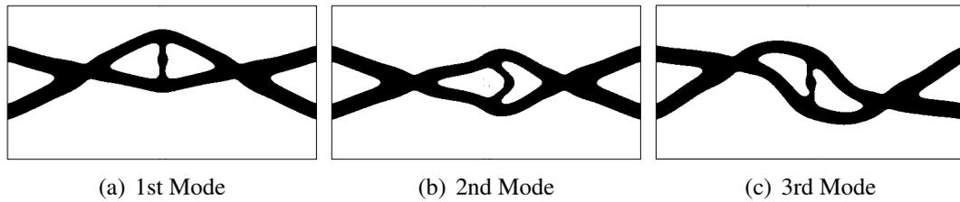
Figure 6: Eigenmodes of the Optimal Configuration
