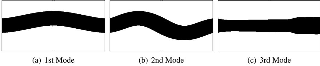
Figure 4: Eigenmodes of the Initial Configuration
