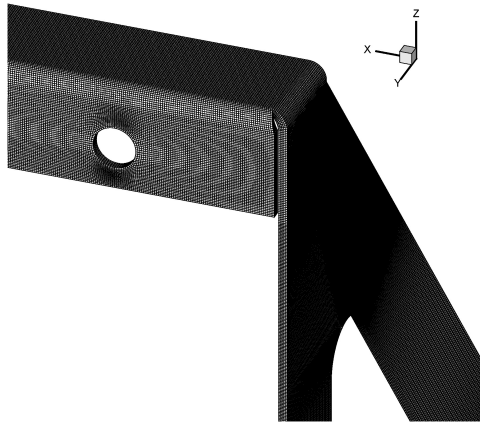
Figure 8: View of the mesh for the bracket
