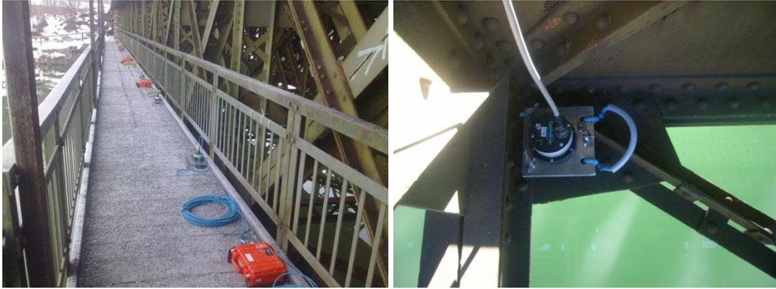
Figure 3: Brimos wireless on the walkway. EpiSensor on the joint.
