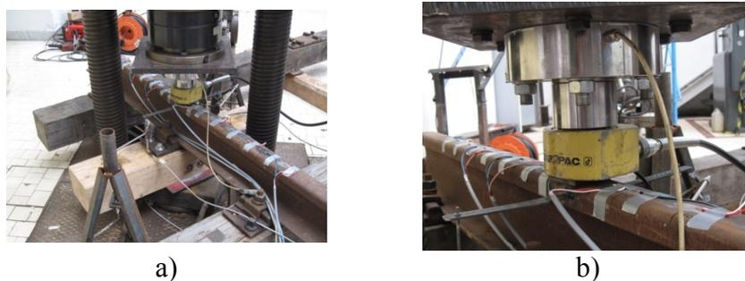
Figure 14: a) global layout of the validation test and b) a particular of the hydraulic jack.
