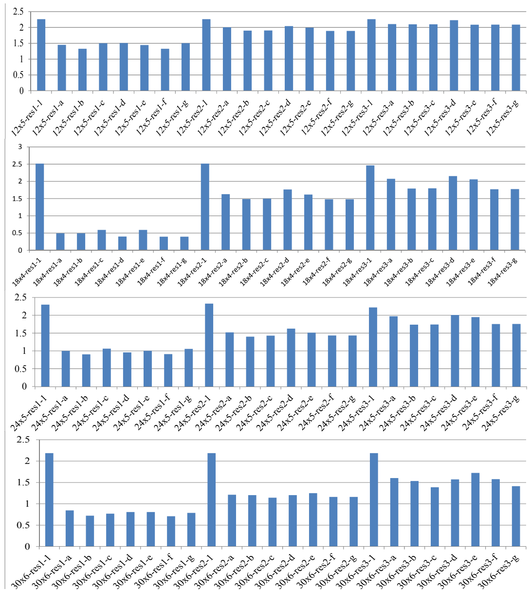
Figure 8. Ultimate load multiplier - GMNIA analysis – accounting for different type of initial imperfections
