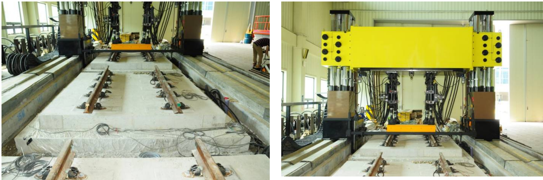
Figure 4: Full-scale loading test of concrete slab track
