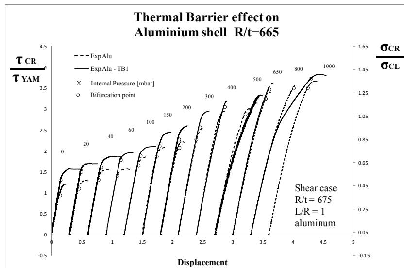
Figure 6. Load displacement response for several internal pressures (0 to 1000 mbars)
