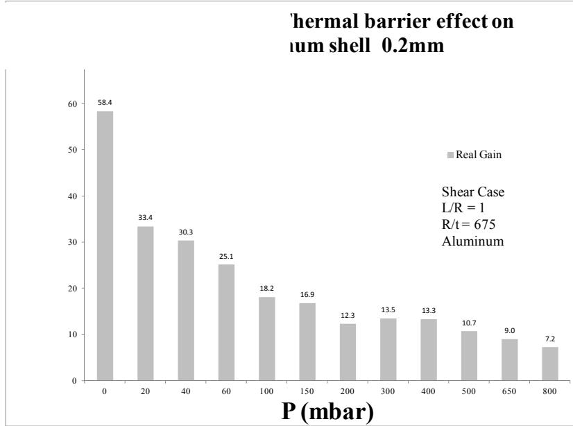
Figure 9. Foam gain compared to non covered shells
