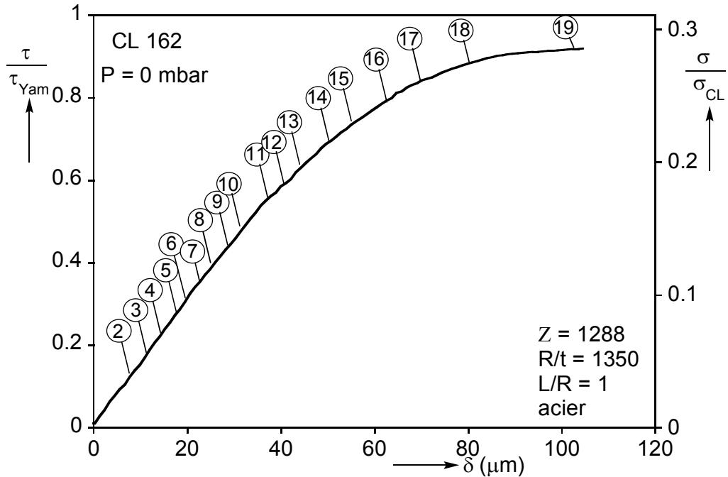
Figure 3: Load displacement curve, CL 162
