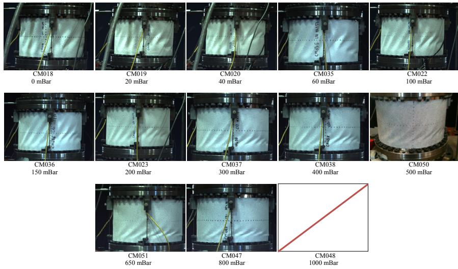
Figure 8. Corresponding covered shells buckling modes (side view)
