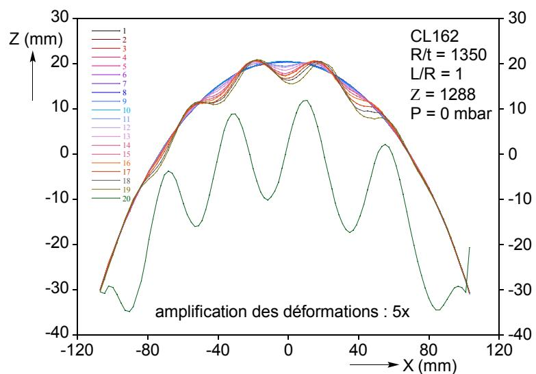
Figure 5: Straight line deformation at cylinder mid-height, CL 162
