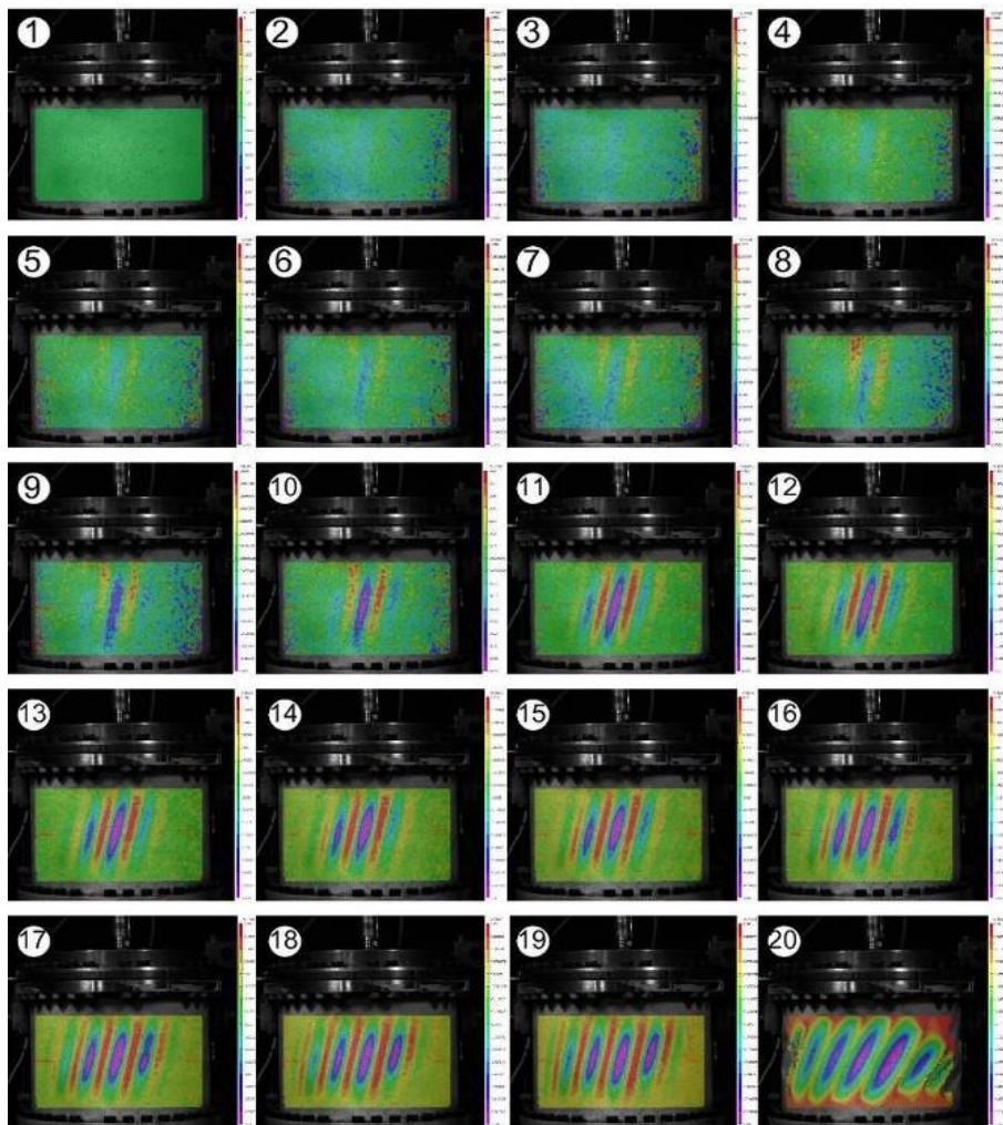
Figure 4: Pictures showing a typical shear buckling experiment conducted on shell CL162 in stainless steel. (VIC 3D)
