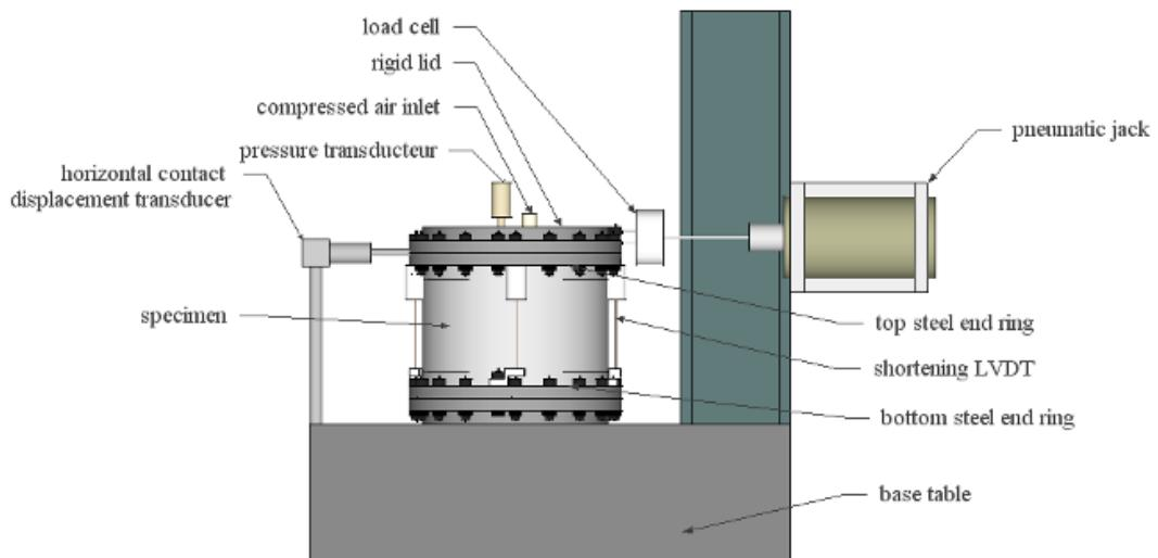
Figure 2: Set up for transverse shear buckling experiments
