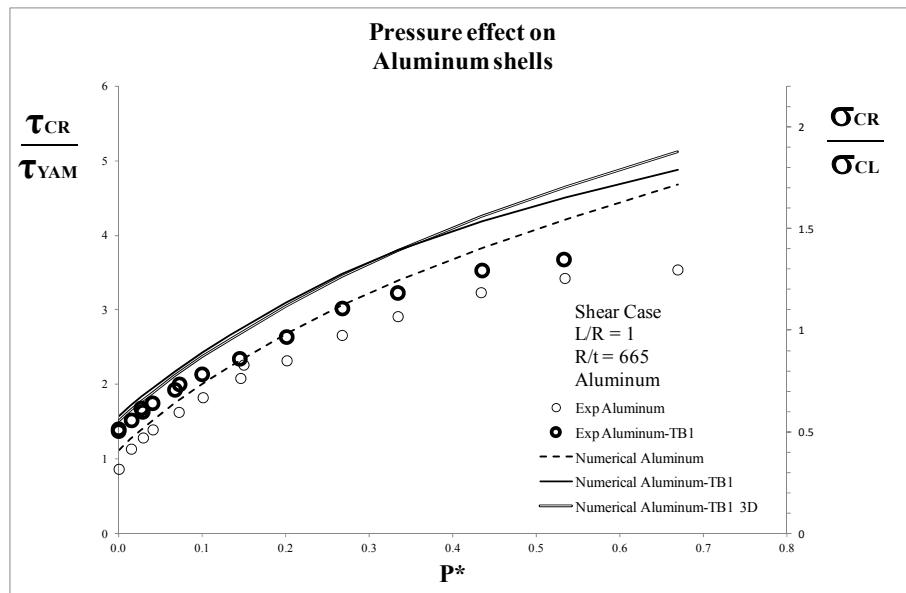
Figure 10. Numerical and Experimental Shear curves,  $R/t = 675$ ,  $L/R = 1$ , aluminum
