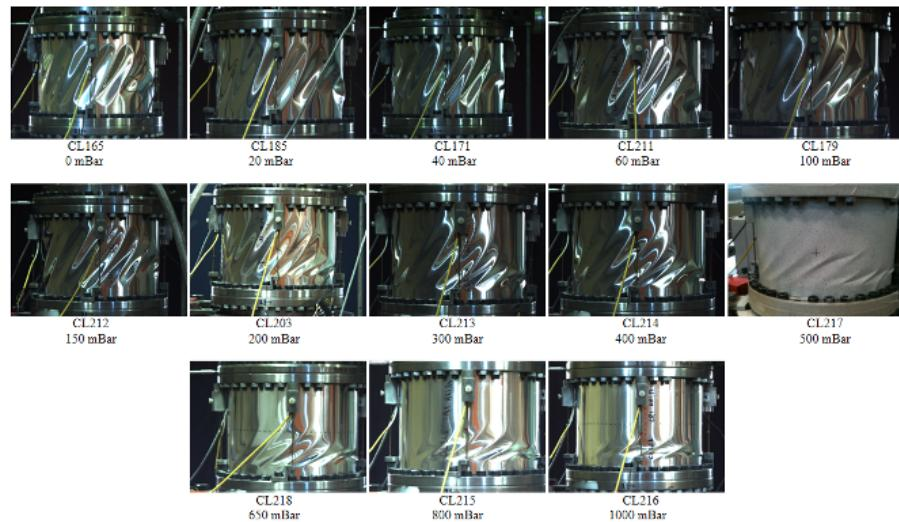
Figure 7. Corresponding non covered shells buckling modes (side view)
