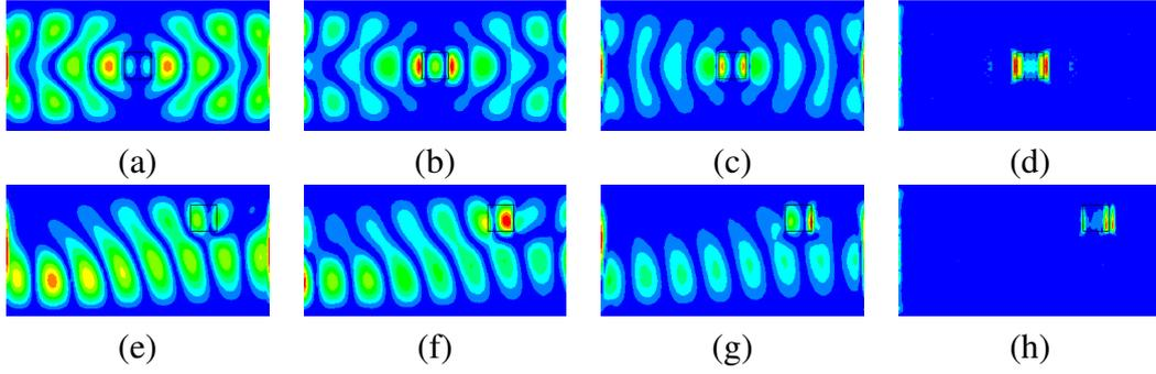
Figure 5:  $DFD_{18}^{(1)}(x, y)$  (a, e),  $DFD_{18}^{(2)}(x, y)$  (b, f),  $DFD_{18}^{(3)}(x, y)$  (c, g) and  $DFD_{18}^{(4)}(x, y)$  (d, h), with the damage at locations L1 (a-d) and L2 (e-h)
