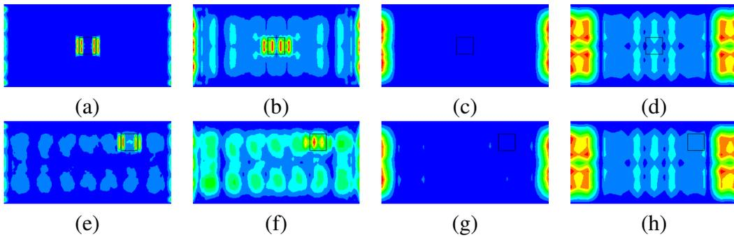
Figure 9:  $SDFD^{(4)}(x, y)$  using model 0 (a, e), model 1 (b, f), model 2 (c, g) and model 3 (d, h), all computed with  $n = 20$ , with the damage at locations L1 (a-d) and L2 (e-h)
