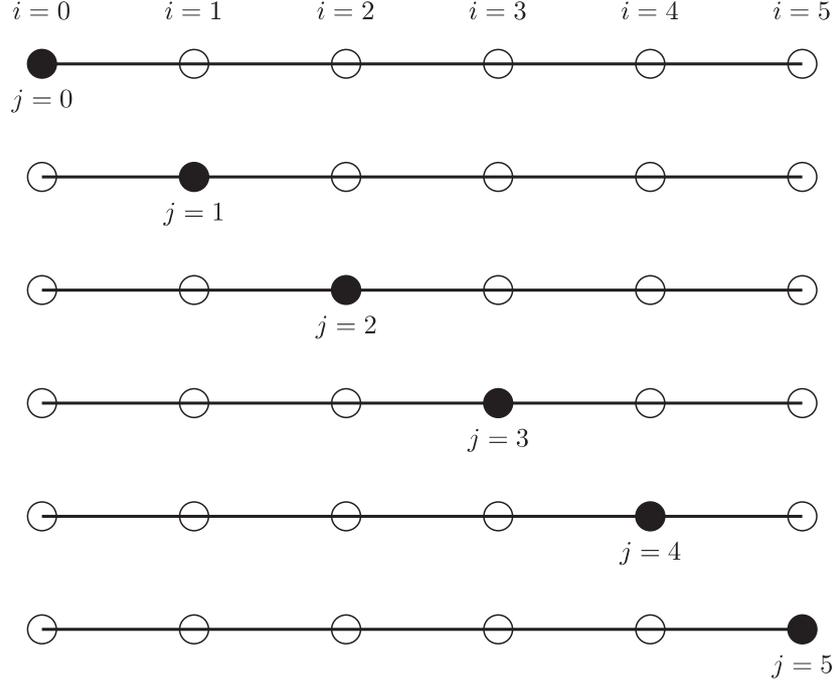
Figure 1: Point where the fourth derivative is computed ● and its neighbouring points ○ using six points finite difference formula
