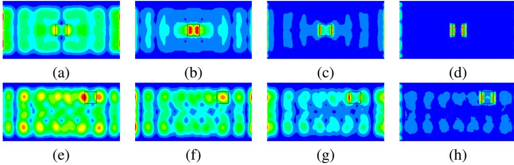
Figure 6:  $SDFD^{(1)}(x, y)$  (a, e),  $SDFD^{(2)}(x, y)$  (b, f),  $SDFD^{(3)}(x, y)$  (c, g) and  $SDFD^{(4)}(x, y)$  (d, h), all computed with  $n = 20$ , with the damage at locations L1 (a-d) and L2 (e-h)
