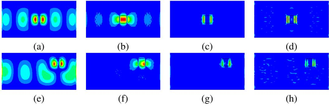
Figure 3:  $DFD_3^{(1)}(x, y)$  (a, e),  $DFD_3^{(2)}(x, y)$  (b, f),  $DFD_3^{(3)}(x, y)$  (c, g) and  $DFD_3^{(4)}(x, y)$  (d, h), with the damage at locations L1 (a-d) and L2 (e-h)
