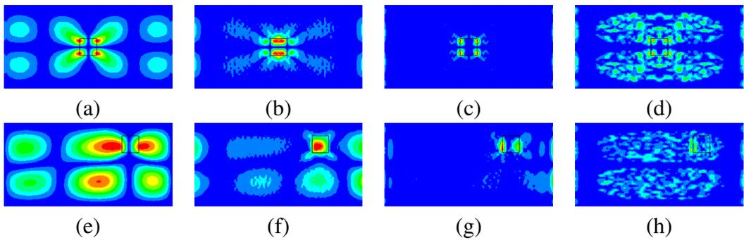
Figure 4:  $DFD_4^{(1)}(x, y)$  (a, e),  $DFD_4^{(2)}(x, y)$  (b, f),  $DFD_4^{(3)}(x, y)$  (c, g) and  $DFD_4^{(4)}(x, y)$  (d, h), with the damage at locations L1 (a-d) and L2 (e-h)
