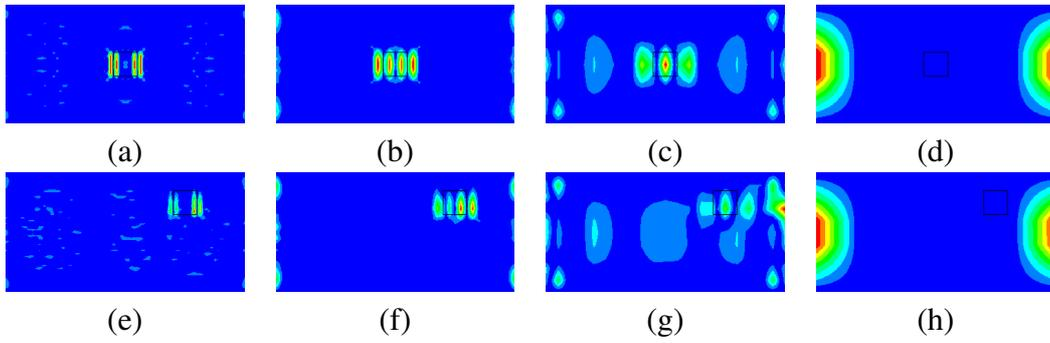
Figure 8:  $DFD_3^{(4)}(x, y)$  using model 0 (a, e), model 1 (b, f), model 2 (c, g) and model 3 (d, h), with the damage at locations L1 (a-d) and L2 (e-h)
