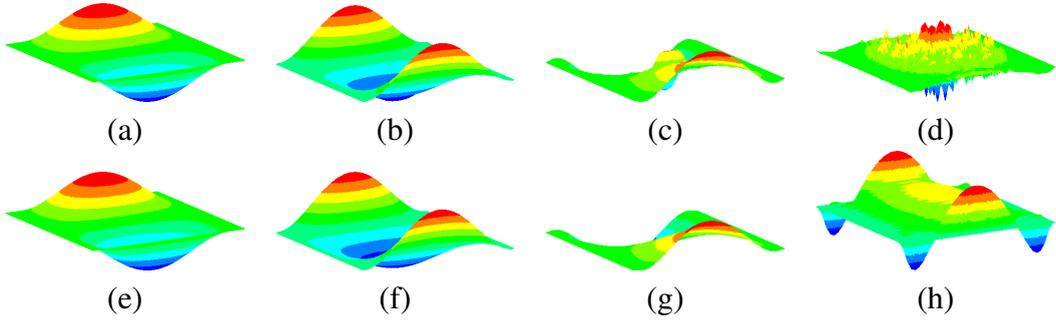
Figure 2: First (a, e), second (b, f), third (c, g) and fourth (d, h)  $x$ -derivative of first mode shape, computed with FEM data (damage location L1) and numerical differentiation (a-d) and the Ritz method data and analytical differentiation (e-h)
