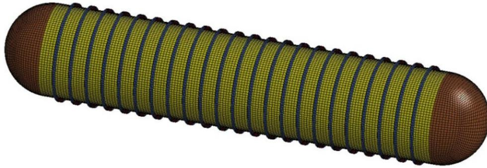
Figure 7: Tee ring-stiffened cylindrical structure
