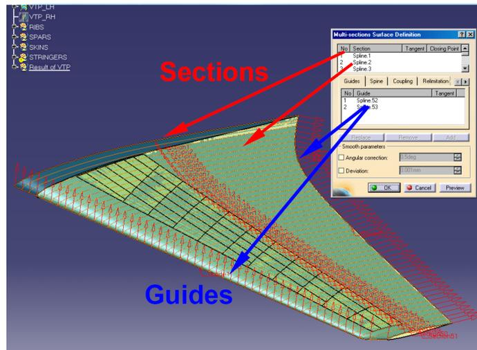
Figure 22: Example of lifting surface and internal structure as generated in CATIA by MARES.
