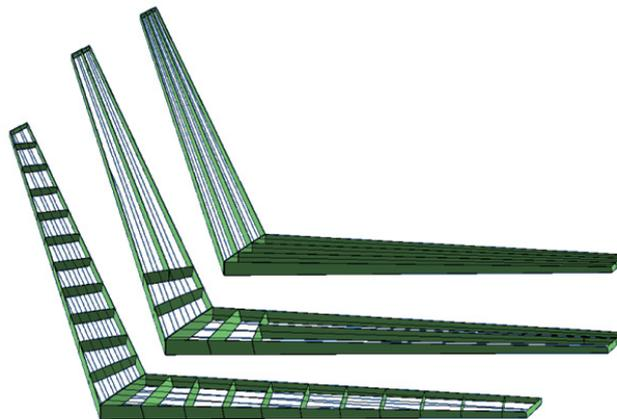
Figure 12: Examples of stringer arrangement
