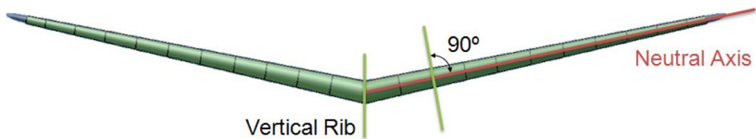
Figure 9: Ribs default orientation
