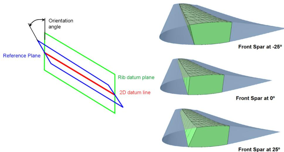
Figure 8: Orientation of rib and spar datum planes
