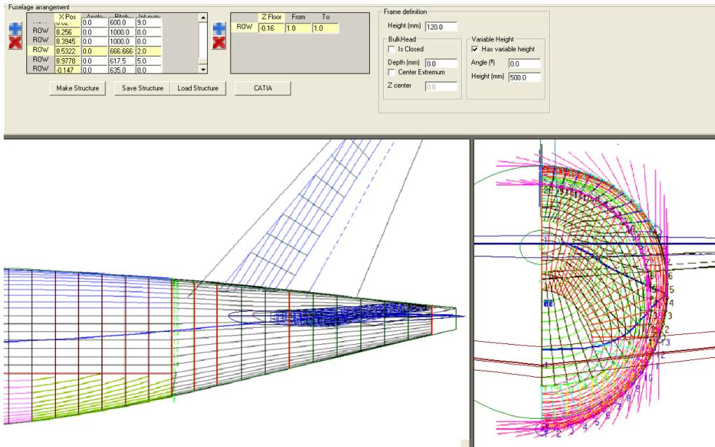
Figure 20: Definition of master frames, floor and window plank lines
