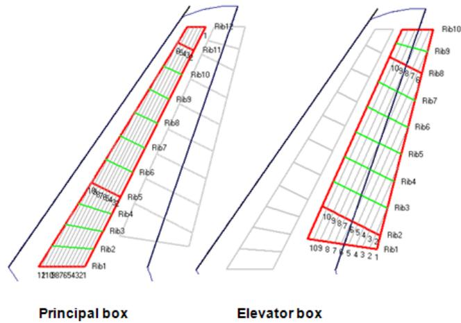
Figure 6: Definition of the structural lay-out for a control surface
