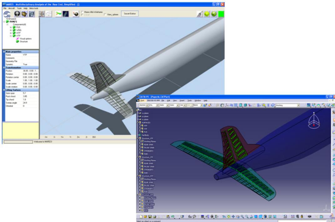
Figure 23: Geometry and structure as rendered in Mares (left) and equivalent CAD model in CATIA V5, generated automatically by MARES (right)
