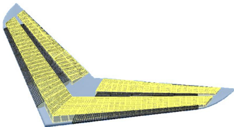
Figure 16: Global FEM of a conventional tailplane rendered in Mares
