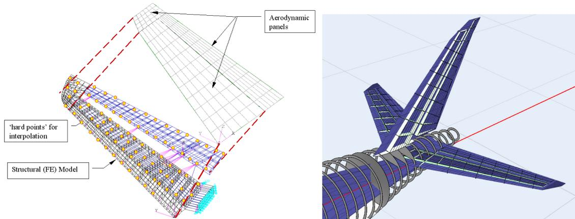
Figure 18: Aeroelastic model for loads generation. Coupling of the DLM mesh with structural hard points (left) and automatically generated aerodynamic mesh on fuselage and tail surfaces (right)
