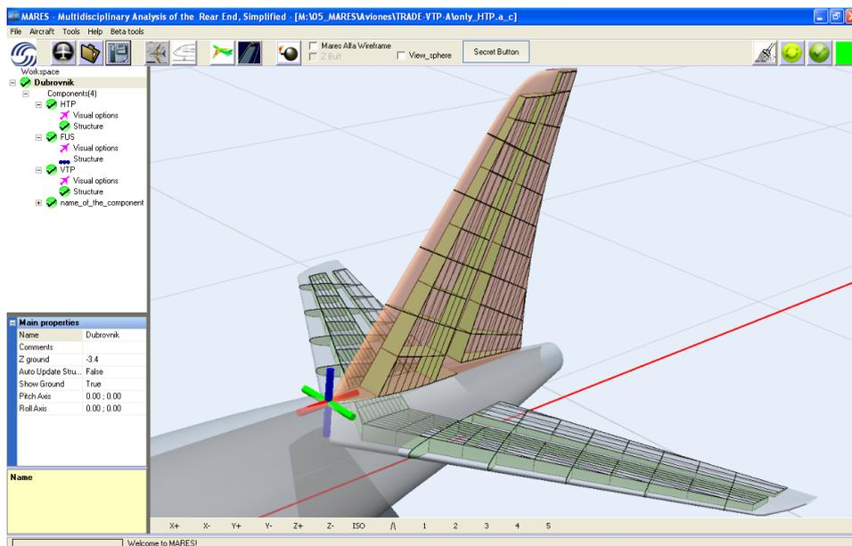
Figure 14: Final structure layout for all rear-end lifting surfaces
