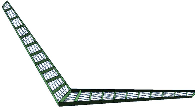
Figure 13: Stringer orientation different on each side of the box
