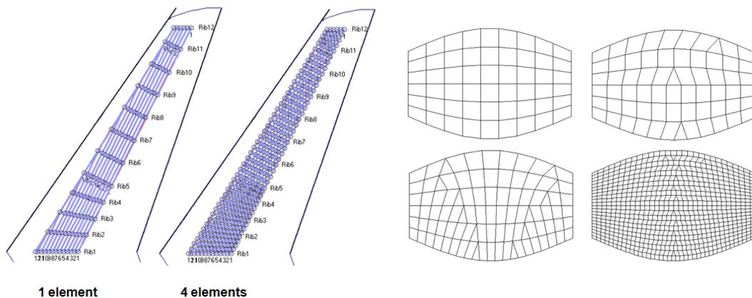
Figure 15: Different number of elements between ribs for the same structural arrangement (left), examples of unstructured "sneaking" meshes for ribs (right)
