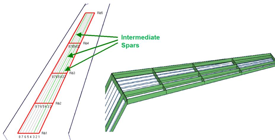
Figure 5: Multi-spar box lay-out definition (left), 3D rendering (right)
