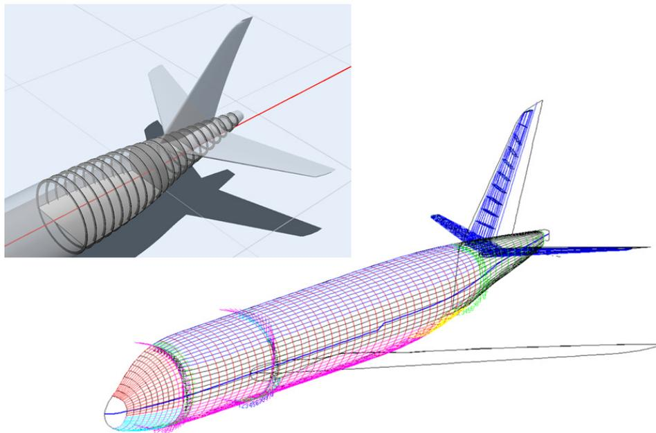
Figure 21: Fuselage structure rendered in MARES (top), FEM mesh topology (right)
