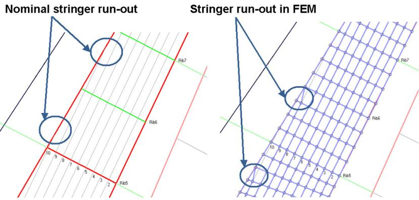
Figure 3: Nominal stringer run-out (left) and modelling of the run-out in a finite elements model (FEM) mesh with intermediate elements in the rib-bay (right)
