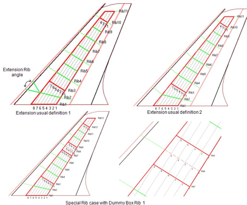
Figure 7: Secondary structure definition
