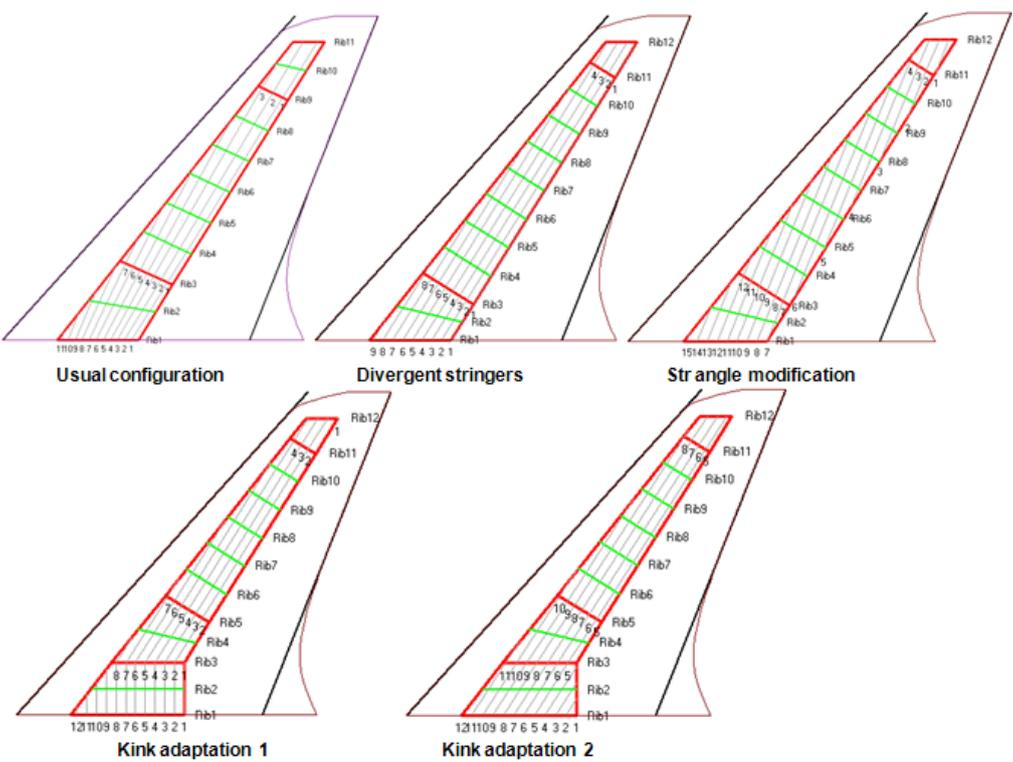
Figure 4: Different stringer lay-out possibilities
