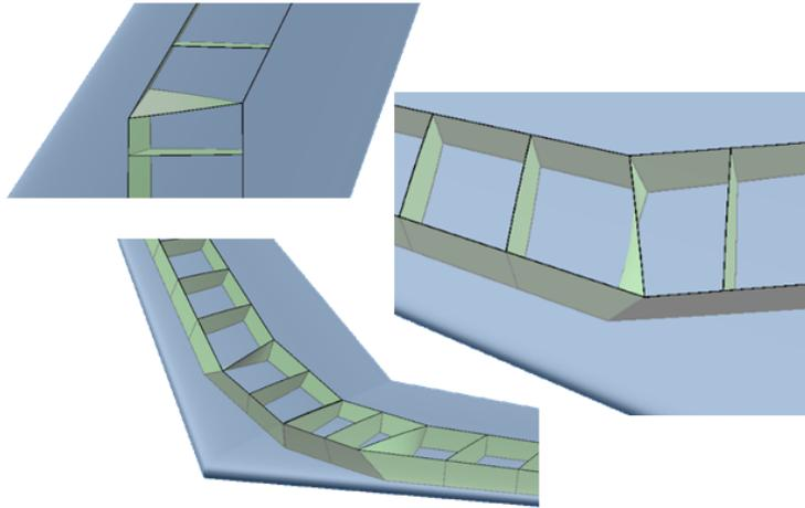
Figure 11: Rib warping at spar kinks
