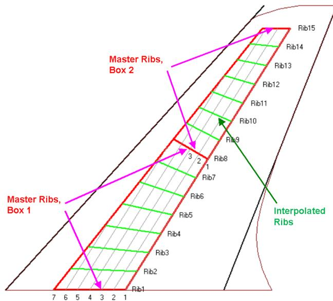
Figure 2: Definition of master ribs and boxes
