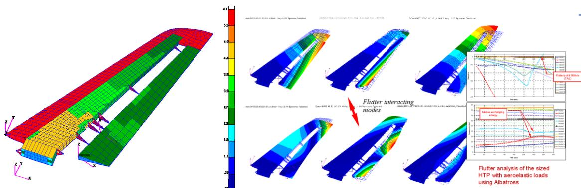
Figure 19: Tailplane structure automatically sized using aeroelastic loads (left). Flutter modes and v-g plot of the sized tailplane (right)
