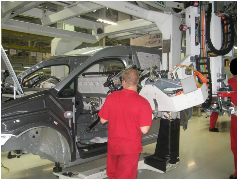
Figure 2: Assembly of the dashboard to the car body with utilization of the industrial manual manipulator
