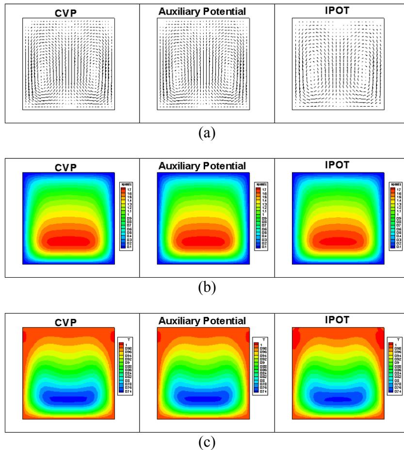
Figure 3: Predictions of the three methods for  $Re=200$ ,  $Pr=0.7$  and  $Gr=100$  at downstream location  $z=10$ . The sets of plots correspond to (a) secondary velocity vector plots, (b) contours of the axial velocity and (c) contours of the temperature.
