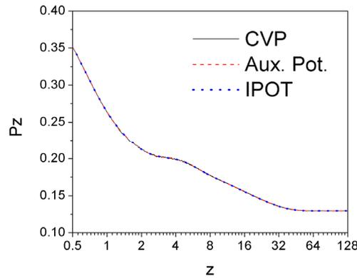
Figure 4: Comparison of the predictions for the axial variation of the absolute value of the axial pressure gradient  $Pz$  for the three methods. The case corresponds to with  $Re=200$ ,  $Pr=0.7$  and  $Gr=100$ .
