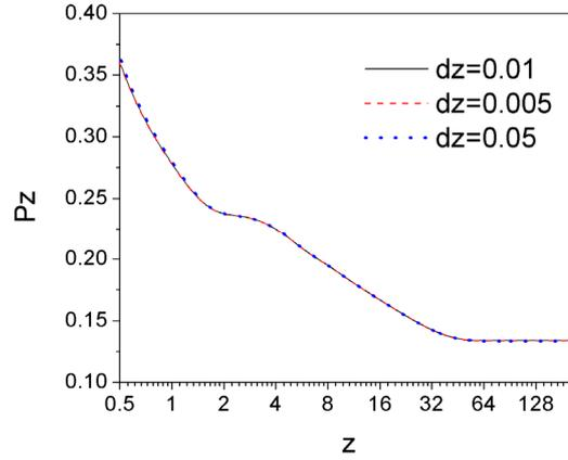
Figure 2: Comparison of the predictions for the axial variation of the absolute value of the axial pressure gradient  $Pz$  for three axial step sizes. The results were obtained with the auxiliary potential method.
