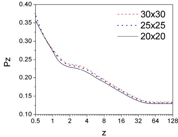
Figure 1: Comparison of the predictions for the axial variation of the absolute value of the axial pressure gradient  $Pz$  for three different grid sizes. The results were obtained with the auxiliary potential method.
