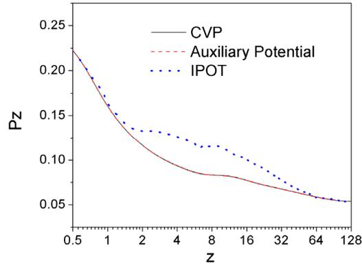
Figure 7: Comparison of the predictions for the axial variation of the absolute value of the axial pressure gradient  $P_z$  for the three methods. The case corresponds to  $Re=500$ ,  $Pr=0.7$  and  $Gr=100$ .
