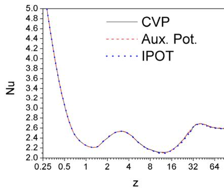
Figure 5: Comparison of the predictions for the axial variation Nusselt number for the three methods. The case corresponds to with  $Re=200$ ,  $Pr=0.7$  and  $Gr=100$ .
