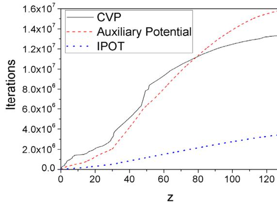
Figure 8: Comparison of total number of iterations of the three methods. The case corresponds to  $Re=200$ ,  $Pr=0.7$  and  $Gr=100$ .
