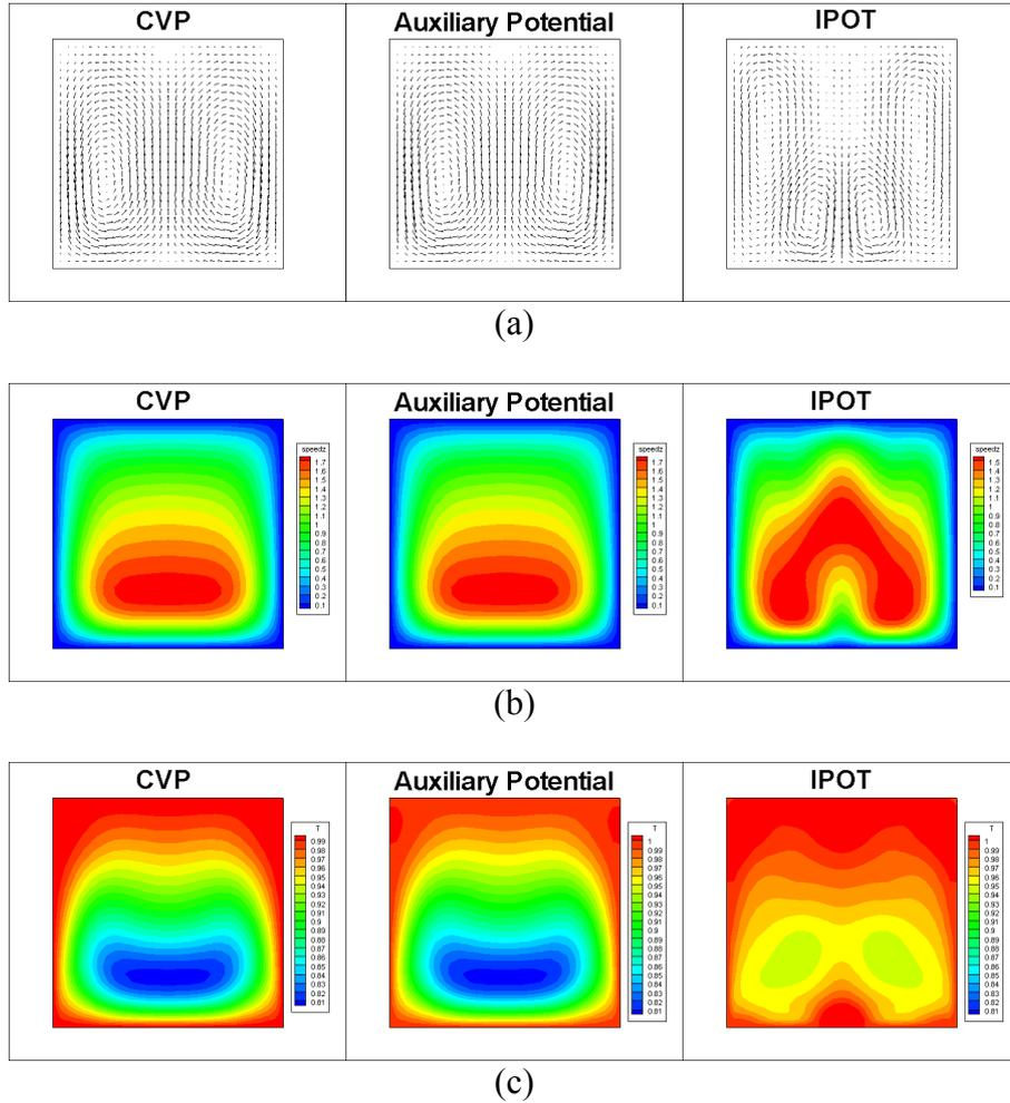
Figure 6: Predictions of the three methods for  $Re=500$ ,  $Pr=0.7$  and  $Gr=100$  at downstream location  $z=30$ . The sets of plots correspond to (a) secondary velocity vector plots, (b) contours of the axial velocity and (c) contours of the temperature.
