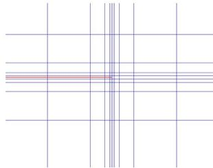
Figure 4: Distribution of elements : whole view and around the crack tip.
