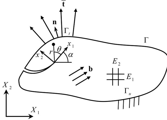
Figure 1: An arbitrary orthotropic cracked body subjected to body force  $\mathbf{b}$  and traction  $\bar{\mathbf{t}}$ .
