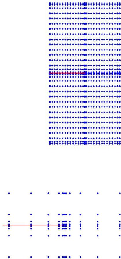
Figure 3: Distribution of control points: whole view and around the crack tip .
