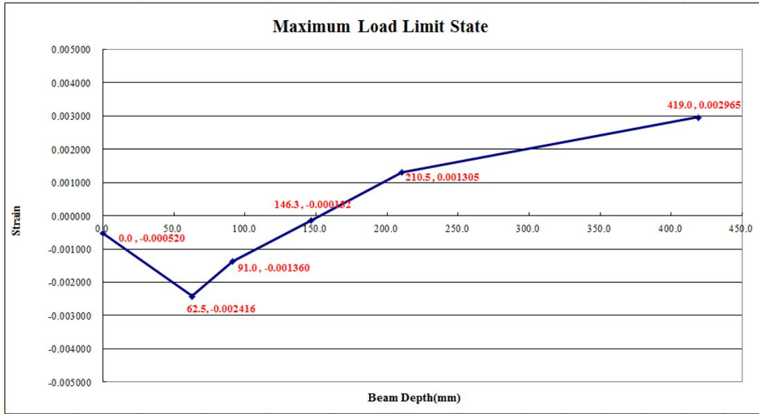
Figure 7: Transition of Strain in Maximum Load Limit State of Specimen #2
