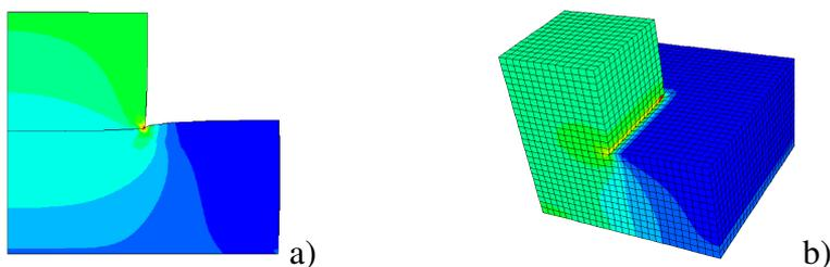
Figure 1: The deformed configurations (a)two-dimensional and (b)three-dimensional.
