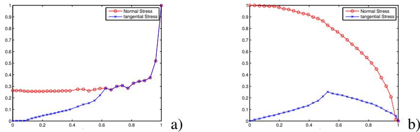
Figure 3: Normalized contact pressures (a) two-dimensional and (b) axisymmetric.
