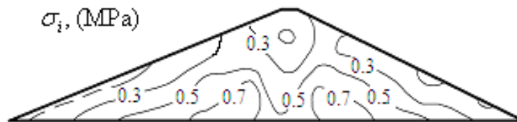
Figure 3: Lines of distribution of the levels of intensity of stresses \sigma_i in the section of Sokh dam
