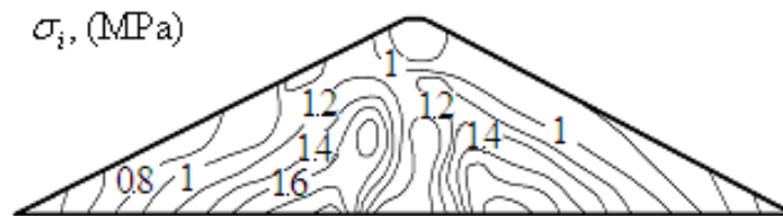
Figure 7: Isolines of maximal values of intensity in the section of a dam ( H=185\text{m} ) at moisture content of soil in a kernel W=10\% )
