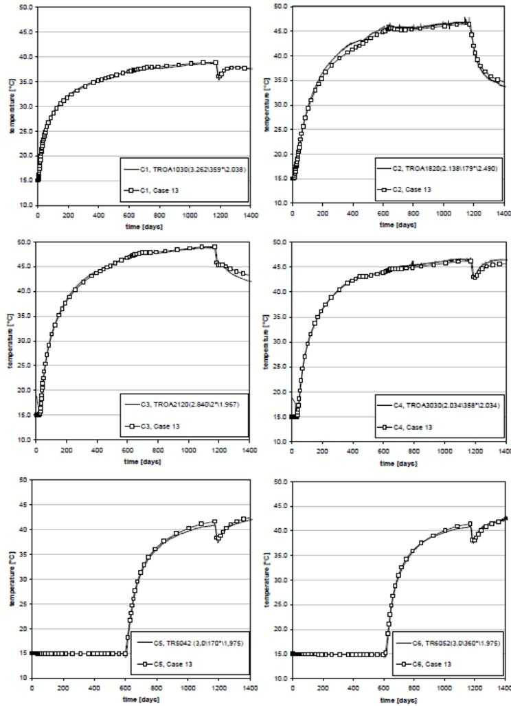
Figure 2: Temperature in sample points approx. at mid height of the canister and 2 m from the canister center, [5].
