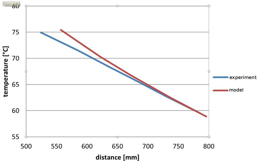
Figure 6: Temperature profiles in the vicinity of the first borehole, November 15, 2004.
