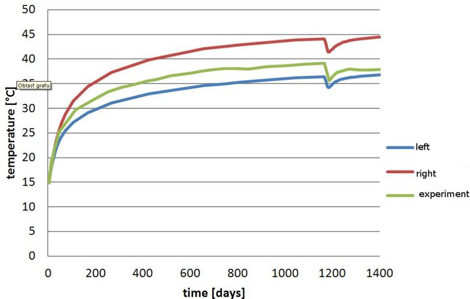
Figure 5: Temperature profiles, left side (blue), right side (red), experiment (green) - first borehole.
