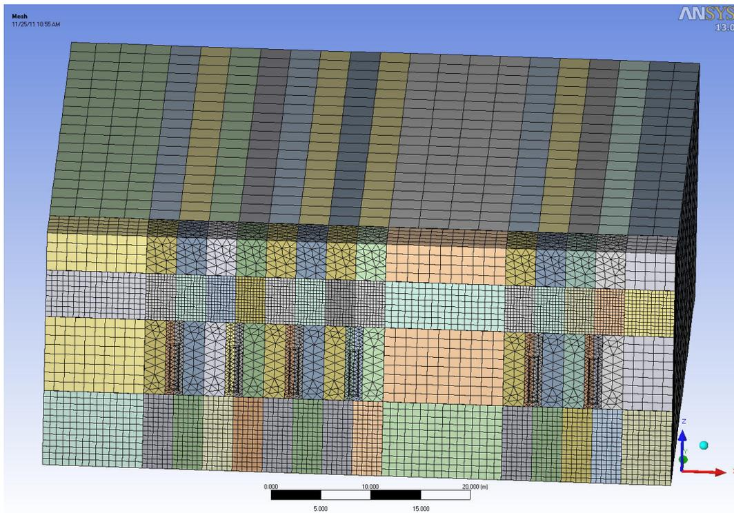
Figure 3: The detail of the finite element mesh of the Prototype Repository model
