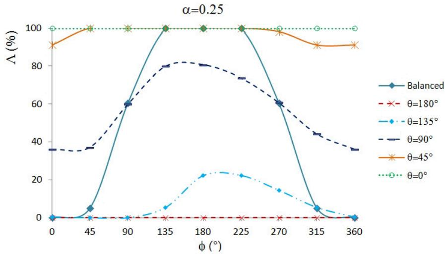
Figure 10: Opening of the crack in a rotation for different eccentricities.  $\alpha=0.25$
