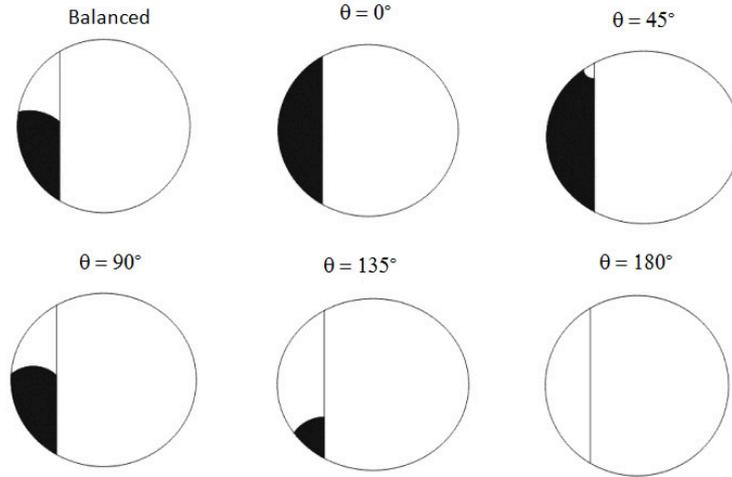
Figure 8: Opening of the crack (in black) for different angles of eccentricity,  $\theta$ . Case  $\phi = 270^\circ$  and  $\alpha=0.25$
