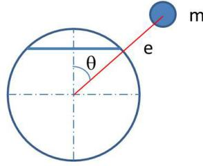
Figure 3: Relative position of the eccentricity
