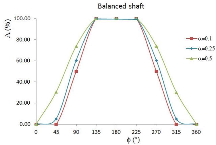
Figure 7: Opening of the crack in a balanced shaft in a rotation for different crack lengths
