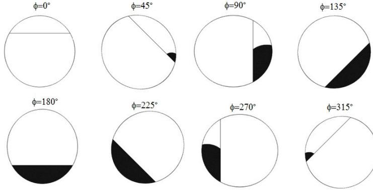
Figure 5: Opening of the crack (in black) for a balanced shaft with  $\alpha=0.25$  in a full rotation
