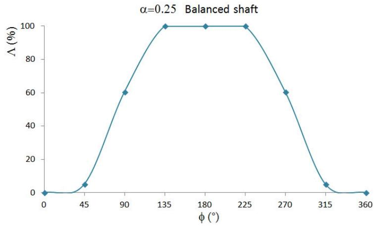
Figure 6: Opening of the crack in a rotation of the balanced shaft
