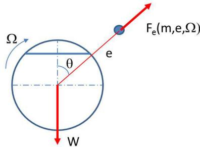
Figure 4: Resume of the applied forces on the shaft
