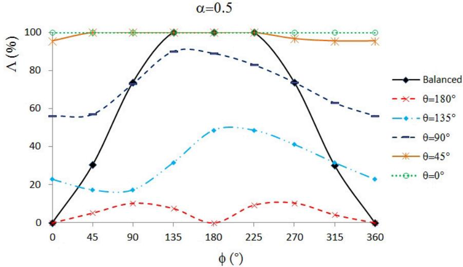
Figure 11: Opening of the crack in a rotation for different eccentricities.  $\alpha=0.5$
