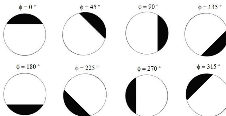
Figure 2: Angular positions of the crack during one rotation
