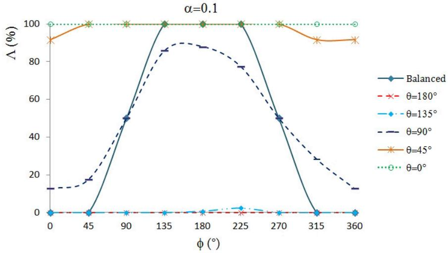
Figure 9: Opening of the crack in a rotation for different eccentricities.  $\alpha=0.1$
