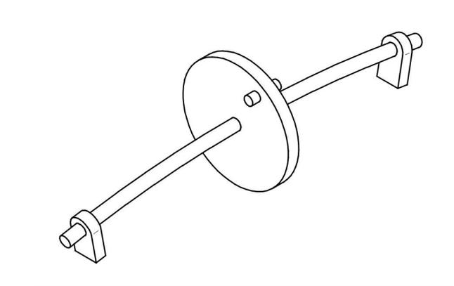
Figure 1: Jeffcott rotor with an eccentric mass.
