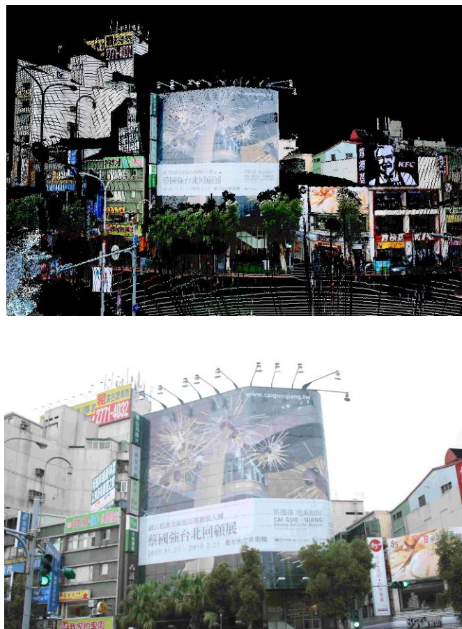
Figure 2. Three-dimensional point cloud (left) and matching photograph (right)
