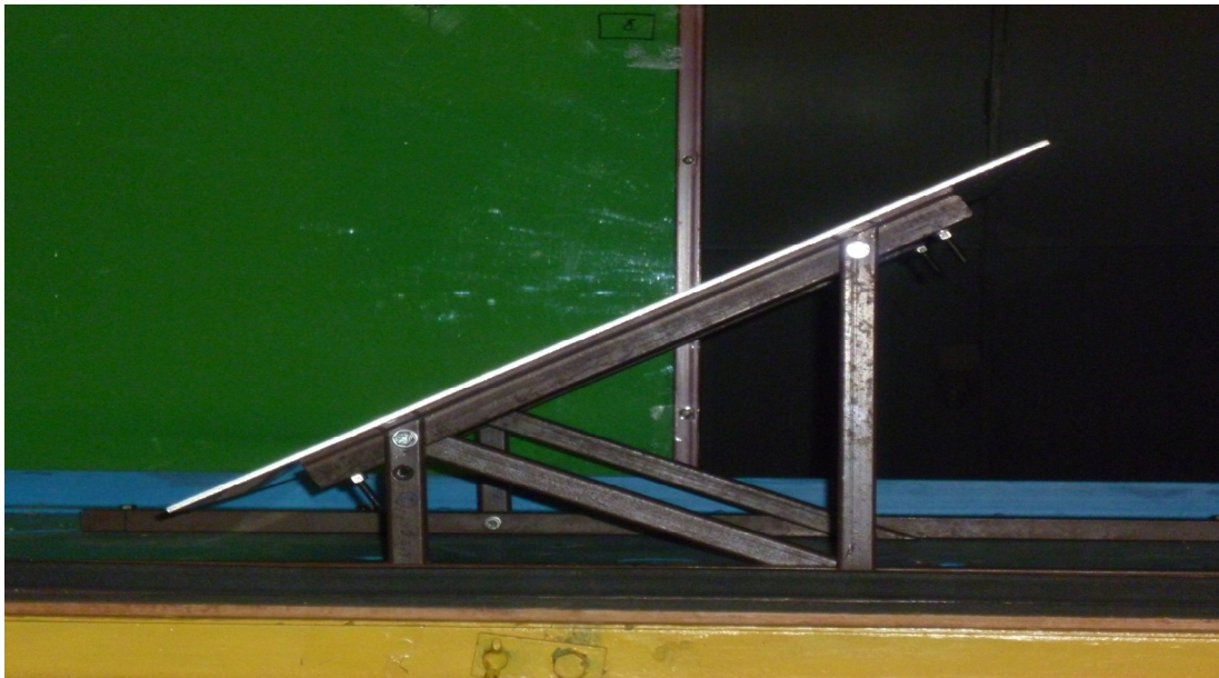
Figure 1. Side view of the skew plate studied in aerodynamic tunnel
